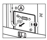
**Warning**: Do not pull on the individual cables at the plug of the control cable (D-A) as this may damage the cable!
