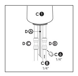
3. Choose a location next to the sink for the 2-way fitting (C-1) so that it can be operated professionally without interfering with the work around the sink. The location you choose should be approx. 4 cm (1.5") from the edge of the sink and approx. 30 cm (11"-12") from the faucet.
