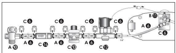
quick-release fastener opening of the water inlet (B-11) on the bottom of the ECAIA ionizer S. Finally, fix the 5 1/4" safety pins (C-6) in place. Afterwards, connect the cable of the solenoid valve (C-12) to the cable plug-in connector on the bottom of the ECAIA ionizer S.
