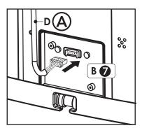
7. Plug the power cable of the ECAIA Ionizer S into the socket. The display on the ECAIA ionizer S is deactivated. The ECAIA ionizer S+ is now only be operable via the buttons on the ECAIA ionizer S faucet.
