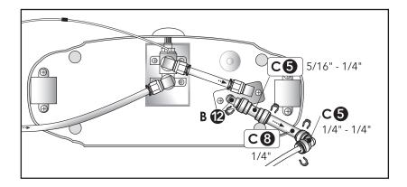
The ECAIA ionizer S can be placed in a lower cabinet or mounted to the wall. To do this, please follow the instructions under point "1.6 - ECAIA ionizer S Wall Mounting" in the complete user manual (long version) for the ECAIA ionizer S.
