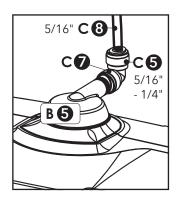
6. Connect the 5/16" to 1/4" quick-release fastener adapter (C-5) to the lower water outlet (B-12) on the device. Connect the 5/16" to 1/4" quick-release fastener adapter (C-5) and the 1/4" quick-release angle adapter (C-5) using the 1/4" outlet hose for acidic water (C-8) as required (5-12cm). Then, connect the 1/4" outlet hose for acidic water (C-8) to the 1/4" quick-release angle adapter (C-5) on the device. Finally, firmly secure the 5/16" safety pin (C-6) and the 3 1/4" safety pins (C-6).
